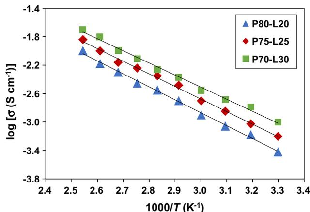
Fig. 3. The variation of logarithm ionic conductivity as a function of inverse absolute temperature from 303 K to 393 K.
