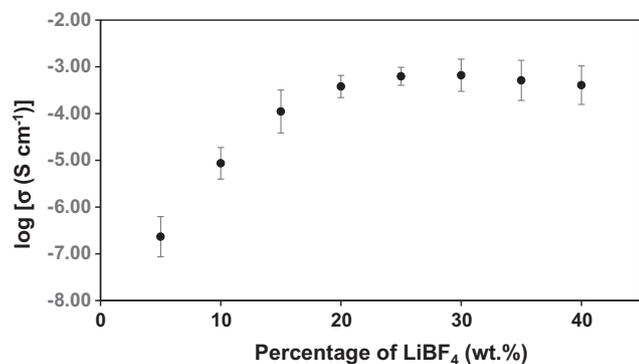
Fig. 2. The variation of ionic conductivity with different lithium salt content in PAA-based electrolyte systems.
