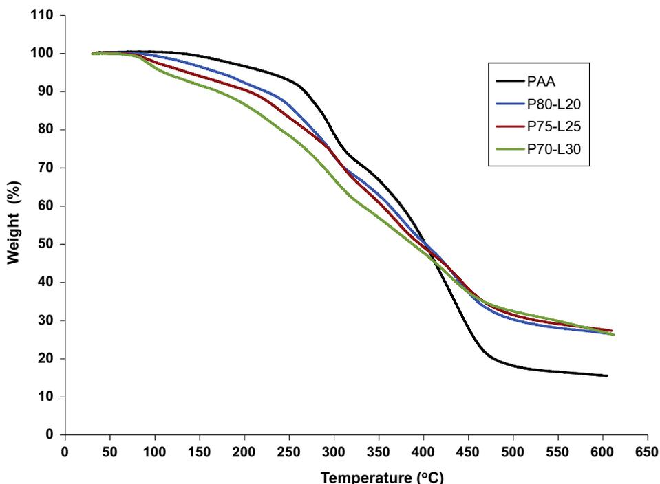
Fig. 8. TGA curves of pure PAA, P70-L30, P75-L25, and P80-L20.
