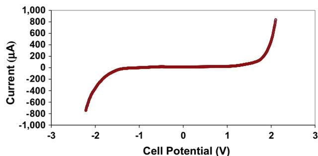
**Fig. 7.** LSV curve of PAA system with 30 wt% LiBF<sub>4</sub> at ambient temperature. (Scan rate:  $5 \text{ mV s}^{-1}$ ).
