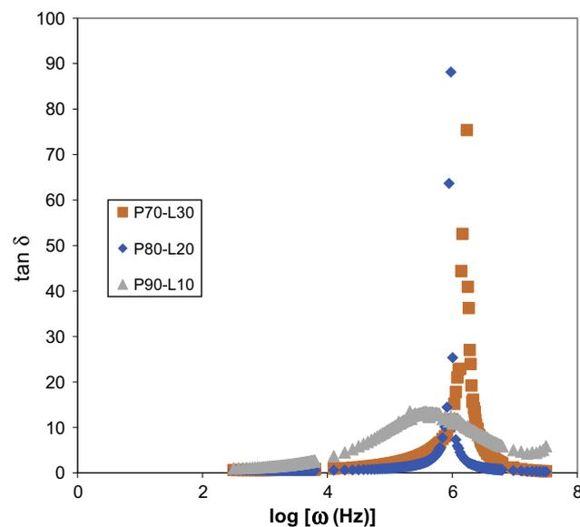
Fig. 5. The frequency dependence variation of loss tangent for P90-L10, P80-L20, and P70-L30.
