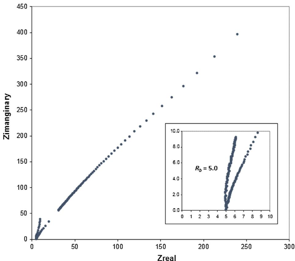
Fig. 1. Cole-Cole plot of PAA-LiBF<sub>4</sub> solid electrolyte films at room temperature. The inset shows the magnified axis of 30 wt% LiBF<sub>4</sub> in a higher frequency region of the real part of complex impedance (x-axis). The imaginary part of complex impedance is the y-axis.
