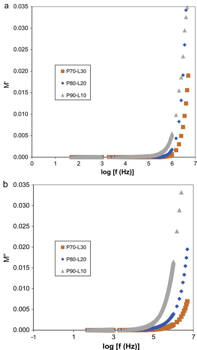
**Fig. 6.** The (a) real part and (b) imaginary part of dielectric moduli as a function of frequency for P90-L10, P80-L20, and P70-L30.
