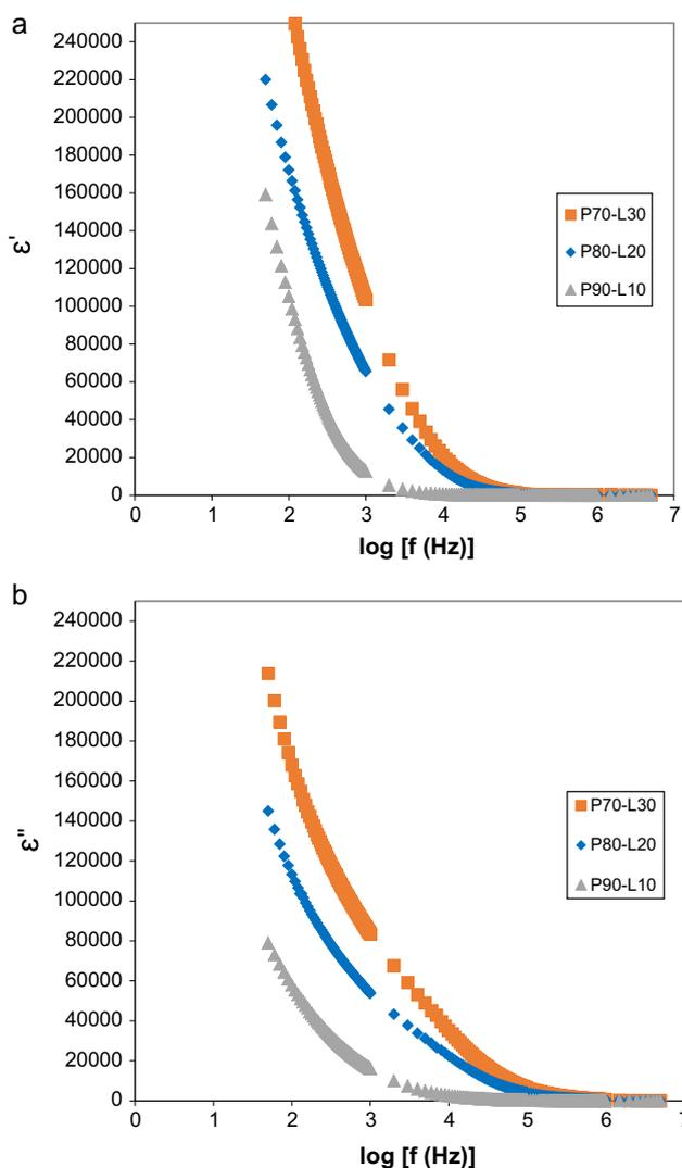
Fig. 4. Variation of (a) dielectric permittivity and (b) dielectric loss for P90-L10, P80-L20, and P70-L30 as a function of frequency at ambient temperature.
