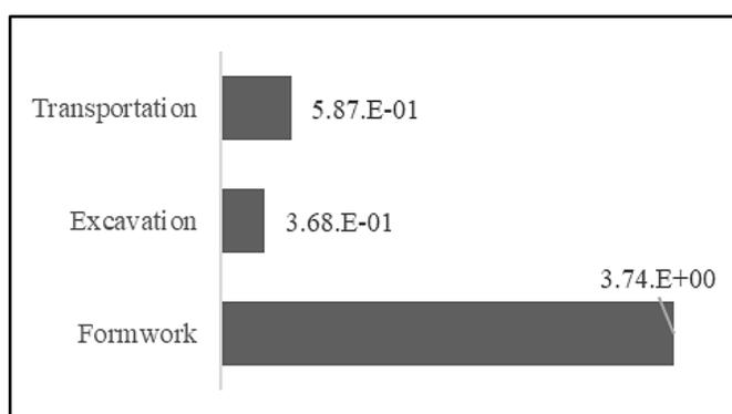
**Figure 4.** LCIA of the building using CML 2001 in the construction phase
