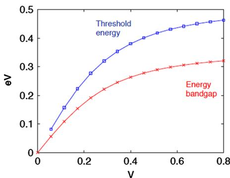
**Fig. 3** Threshold energy and energy bandgap of BLG versus interlayer potential
