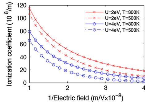
**Fig. 4** Ionization coefficient of BLG versus electric field (including high ranges) for two values of interlayer potential energies and temperatures
