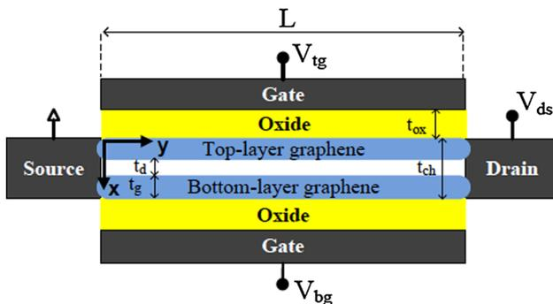
**Fig. 1** Cross sectional view of bilayer graphene double gate transistor
