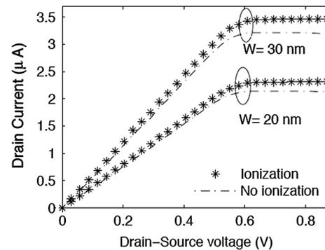
**Fig. 8** Drain current with and without considering the generation rate as a function of drain-source voltage for different channel width
