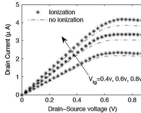
**Fig. 7** Drain current with and without considering the generation rate as a function of drain-source voltage for different values of back gate voltages
