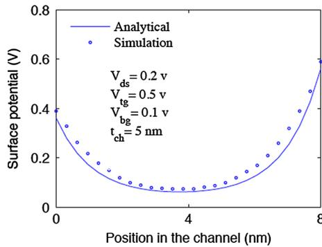
**Fig. 6** The front side ( $x = 0$ ) potential distribution along the channel for channel width comparable with channel length, with  $t_{ox} = 1$  nm,  $L = 8$  nm,  $N_D = 1 \text{ e}^{12} \text{ cm}^{-2}$ ,  $n_i = 1 \text{ e}^{13} \text{ cm}^{-2}$
