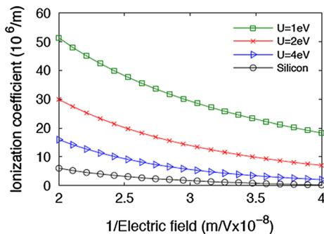
**Fig. 2** Ionization coefficient of BLG versus low range electric field for three different interlayer potential energies. The simulation results of silicon are extracted from Fig. 5 of [25]
