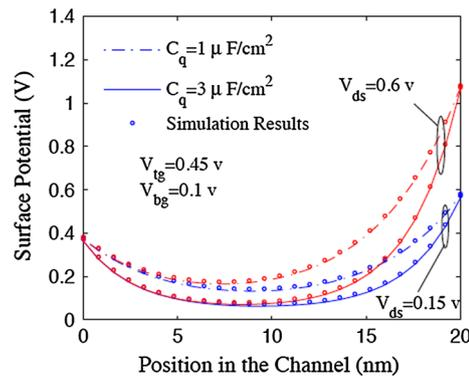
**Fig. 5** Analytical and simulation results of the front side ( $x = 0$ ) potential distribution along the channel with  $t_{ox} = 1$  nm,  $L = 20$  nm,  $N_D = 1 \times 10^{12} \text{ cm}^{-2}$ ,  $n_i = 1 \times 10^{13} \text{ cm}^{-2}$ . The obtained results of the analytical model are represented by lines and the FlexPDE simulation results are represented by symbols
