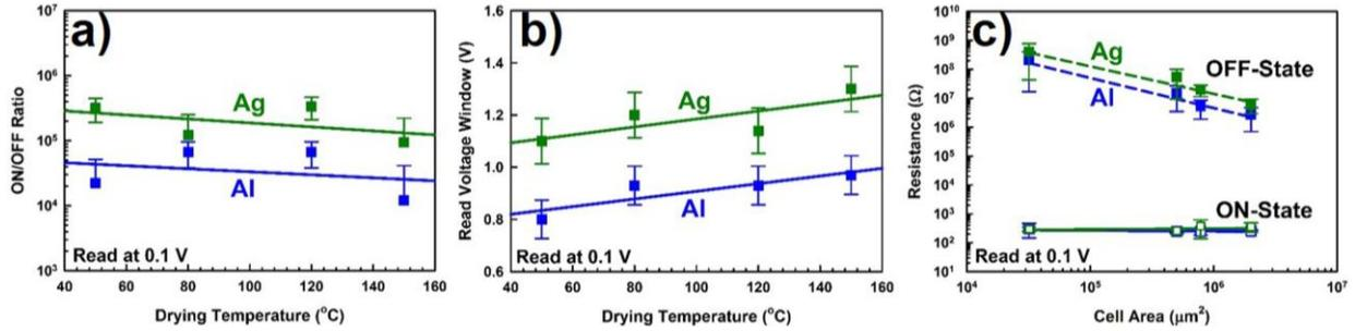
**Figure 2.** Effects of drying temperature of the Aloe vera films on a) ON/OFF ratio and b) read voltage range of the device. c) Cell area dependency of the ON- and OFF-state resistances.
