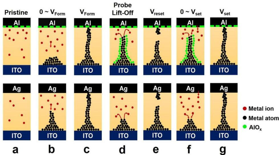
**Figure 3.** Schematics illustrating the resistive switching behavior a) in a pristine device, b) when a voltage is applied on the top electrode, c) forming process, d) probe lift-off incident, e) reset process, and f,g) set process.
