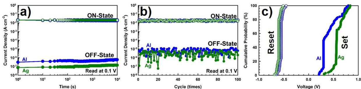
**Figure 4.** a) Data retention characteristics of the device under a continuous 0.1 V voltage stress and b) endurance performance of the device over 100 ON/OFF cycles. c) Cumulative probability distribution of operating voltages for set and reset processes.
