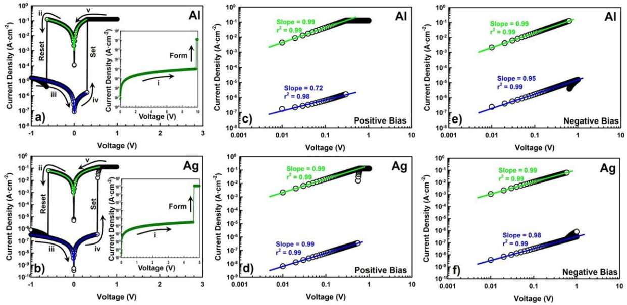
**Figure 1.** Typical  $J$ - $V$  characteristic curves of the a) ITO/Aloe vera/Al and b) ITO/Aloe vera/Ag device. Insets show the initial forming process of the corresponding device. Arrows indicate the direction of voltage sweeps and their sequence is numbered using Roman numerals. Log-log plot of the  $J$ - $V$  characteristics in b,c) positive bias and e,f) negative bias regions of the corresponding device. Solid lines are linear fittings of Ohm's law to the experimental data.
