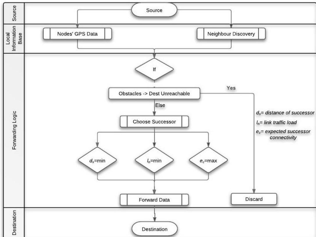
**Fig. 4:** VANET Routing Stepwise Approach
