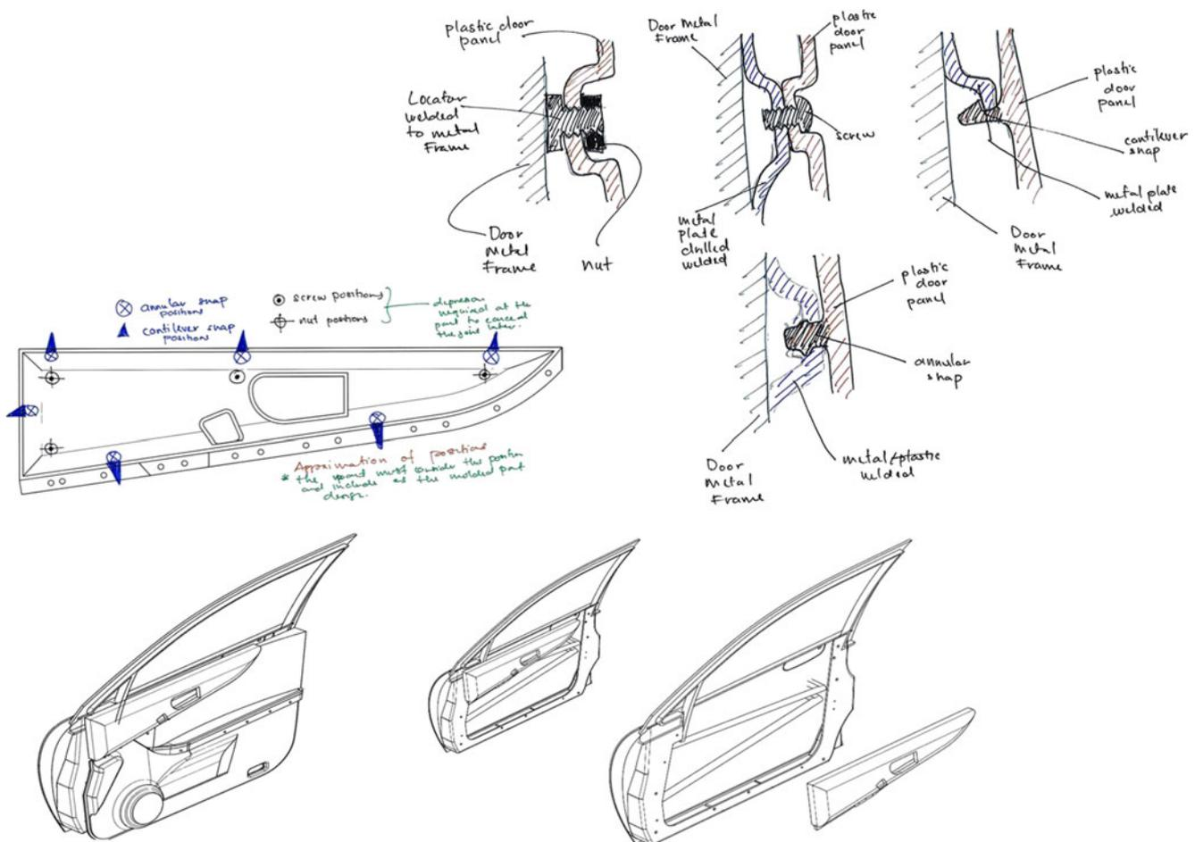
Fig. 3 Initial CAD model of door and sketches of the fastening concept alternatives during conceptual design
