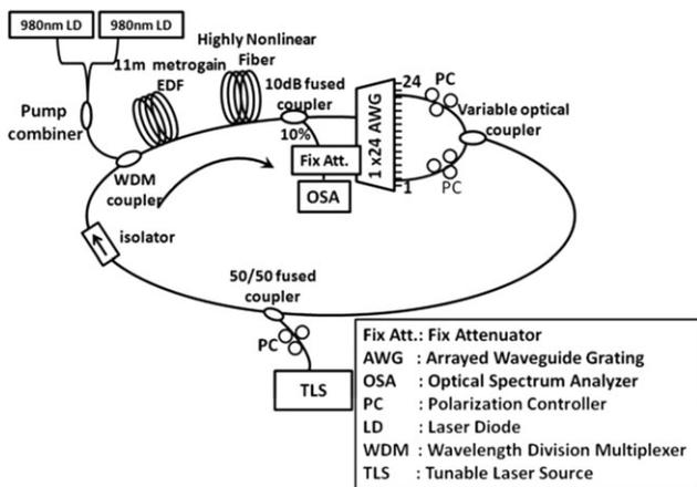
**Figure 1** Schematic diagram for generating FWM effect in a highly nonlinear fiber using dual-wavelengths fiber laser incorporating AWG as a tuning element
