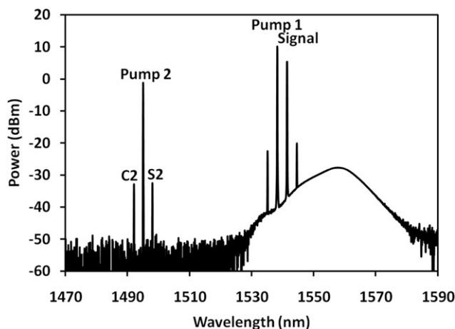
**Figure 3** The typical output spectra at pump 1, signal and pump 2, as well as their converted signals (sideband fields) C2 and S2 when wavelength of pump 1, signal and pump 2 are 1538.3, 1541.5, and 1530 nm
