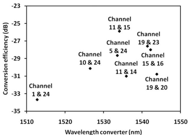
**Figure 2** The value of FWM conversion efficiency for different AWG's channels
