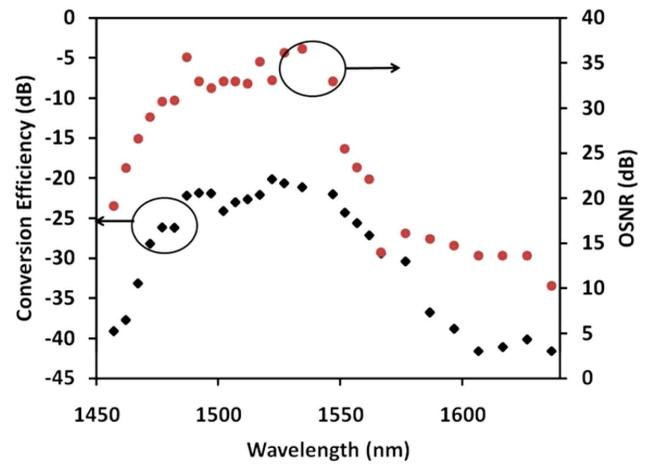
**Figure 5** The conversion efficiency and the OSNR against the converted wavelength. [Color figure can be viewed in the online issue, which is available at [wileyonlinelibrary.com](http://wileyonlinelibrary.com)]
