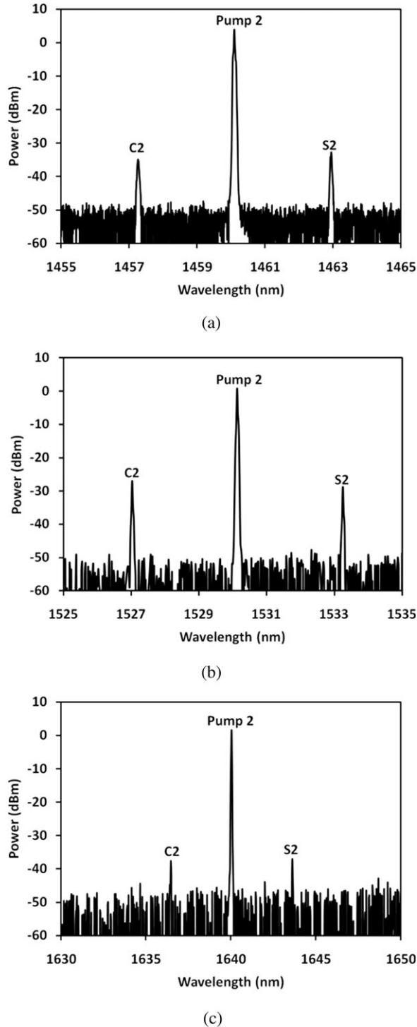
**Figure 4** The output spectra of S2, Pump 2 and C2 when the wavelength of Pump 1 and signal are 1538.3 and 1541.5 nm; (a) Pump 2 is 1460 nm and their input power is 3.86 dBm; (b) Pump 2 is 1530.2 nm and their input power is 3.00 dBm; (c) Pump 2 is 1640 nm and their input power is 3.36 dBm
