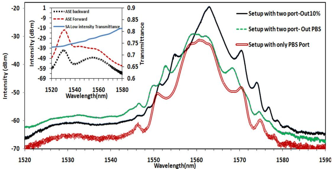
**Figure 3** Spectra measured at different output ports for a ring cavity with 4 m long EDF (DF1500L). Pump power is fixed at 100 mW. Inset shows ASE spectra in forward and backward schemes and also transmittance spectrum (%) of SA. [Color figure can be viewed in the online issue, which is available at [wileyonlinelibrary.com](http://wileyonlinelibrary.com)]
