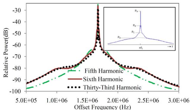
**Figure 8** Typical spectra of different harmonics as a function of the scaled offset frequency for a sub-picosecond pulse train at output port of PBS. The RBW in RFSA is fixed at 3 kHz. Inset shows the noise structure and marks  $P_A$ ,  $P_B$ ,  $P_C$ , and  $P_D$ . [Color figure can be viewed in the online issue, which is available at [wileyonlinelibrary.com](http://wileyonlinelibrary.com)]
