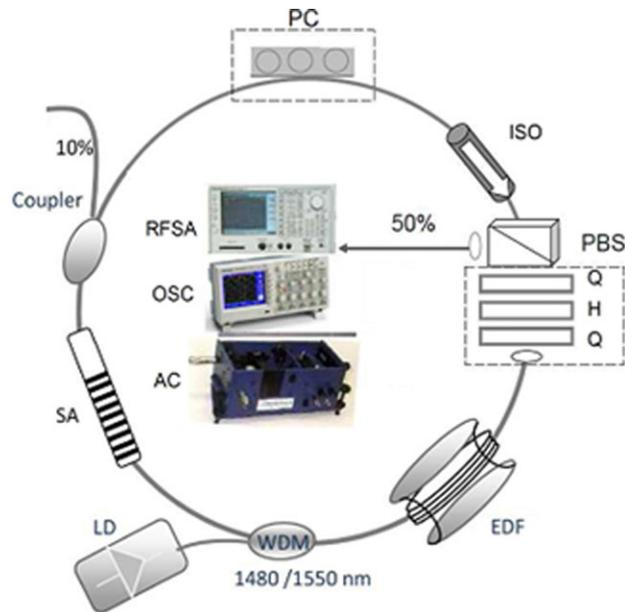
**Figure 1** Experimental setup of the laser EDFL. “WDM: wavelength division multiplexer; SA: saturable absorber; OSC: oscilloscope; RFSA: RF spectrum analyzer; OSA: optical spectrum analyzer; AC: auto-correlator; PC: polarization controller; PBS-isolator: polarizing beam splitter integrated with isolator; H: (zero order)1/2-wave retarder; Q: (zero order) 1/4-wave retarder; ISO: isolator.” [Color figure can be viewed in the online issue, which is available at wileyonlinelibrary.com]
