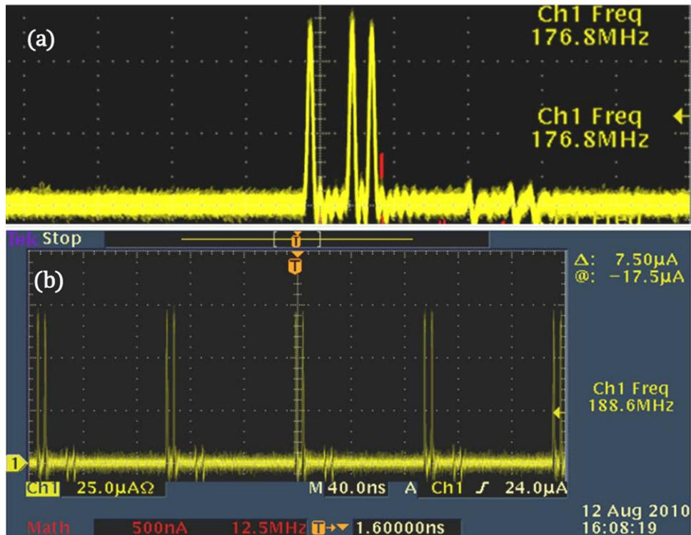
**Figure 5** Period-doubling of multiple vector solitons: (a) Two vector solitons, (b) three vector solitons. [Color figure can be viewed in the online issue, which is available at [wileyonlinelibrary.com](http://wileyonlinelibrary.com)]
