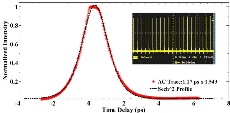
**Figure 4** Autocorrelation trace and pulse train (inset) of the 1.17 ps pulses. Dashed curve: sech<sup>2</sup> fit. Inset pulse train of passive mode locked laser with repetition rate of 9.87 MHz. [Color figure can be viewed in the online issue, which is available at [wileyonlinelibrary.com](http://wileyonlinelibrary.com)]
