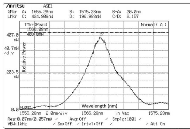
**Figure 9** Spectrum measured at PBS port for an optimal setting
