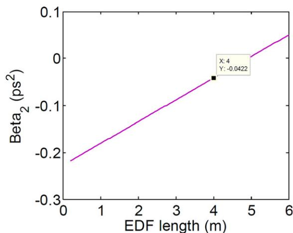
**Figure 2** Net cavity dispersion for various lengths of EDF in the cavity. The total length of cavity is fixed at 10.4 m. [Color figure can be viewed in the online issue, which is available at wileyonlinelibrary.com]
