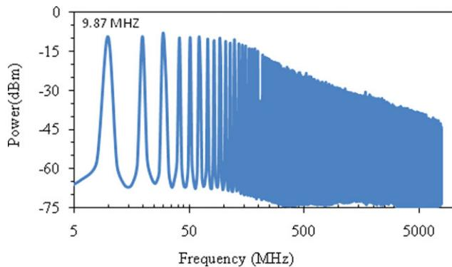
**Figure 7** RF spectrum of pulse train for proposed oscillator without multiple pulsing. The frequency axis in this figure is logarithmic. [Color figure can be viewed in the online issue, which is available at [wileyonlinelibrary.com](http://wileyonlinelibrary.com)]
