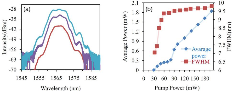
**Figure 6** (a) Spectra measured at PBS port, (b) the variation of the spectral width, and output power as a function of the pump power at the PBS port. [Color figure can be viewed in the online issue, which is available at [wileyonlinelibrary.com](http://wileyonlinelibrary.com)]
