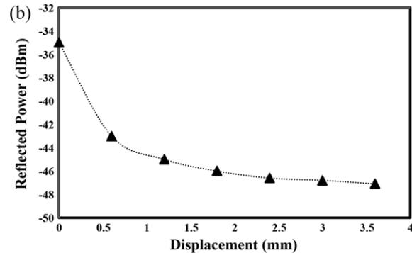
Fig. 6. Output spectra characteristics: (a) output spectra at various displacement of reflector from micro-ball lens and (b) reflected power against the displacement.
