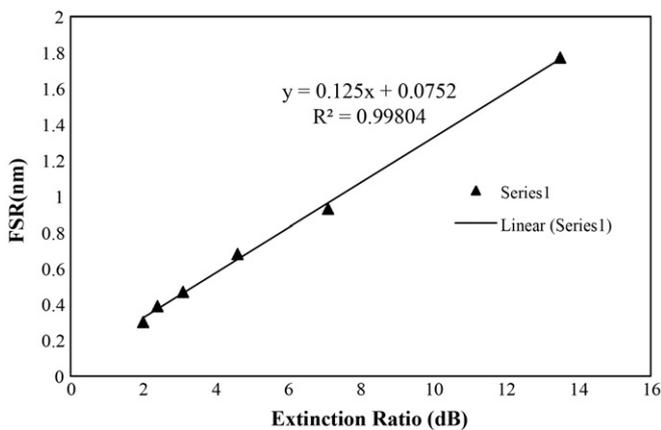
Fig. 8. Linear relationship between FSR and extinction ratio of the output comb of the sensor.
