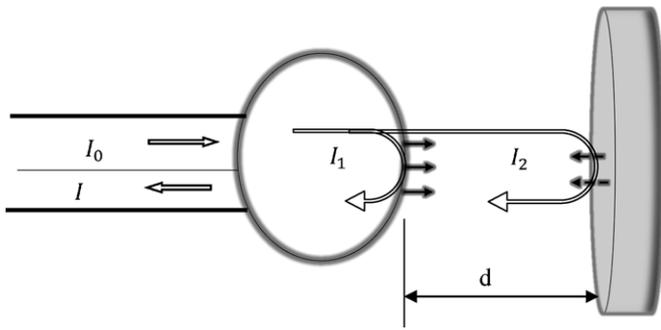
Fig. 4. Schematic diagram showing the light propagation inside the sensor probe and the reflector.
