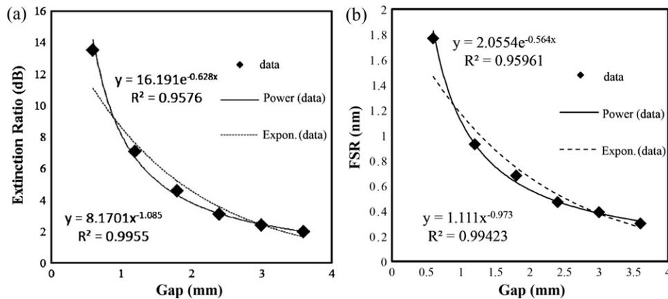
Fig. 7. (a) Extinction ratio and (b) FSR against the displacement.
