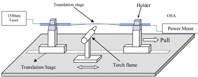
Fig. 1. Microfiber coupler fabrication setup.
