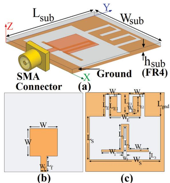
**Figure 1** Geometry of the proposed microstrip-fed slot antenna, (a) side view, (b) bottom view, and (c) top view. [Color figure can be viewed in the online issue, which is available at [wileyonlinelibrary.com](http://wileyonlinelibrary.com)]
