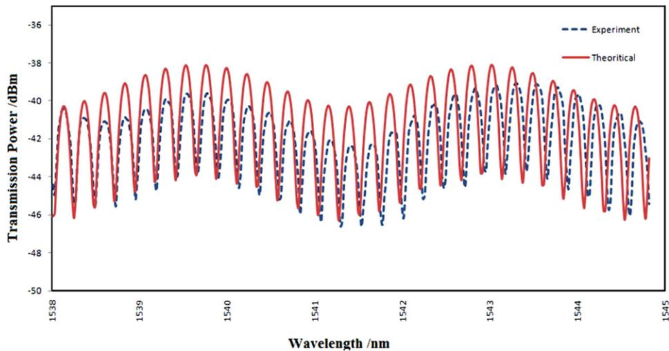
**Figure 3** The resonant spectrum of the proposed microfiber hybrid structures obtained from the experiment and theoretical analysis. [Color figure can be viewed in the online issue, which is available at [wileyonlinelibrary.com](http://wileyonlinelibrary.com)]
