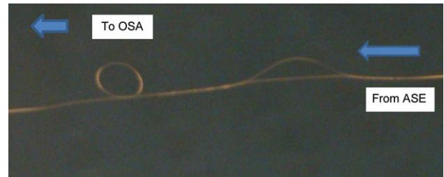
**Figure 2** Microscope image of the microfiber hybrid structure consisting of MMZI and MKR. [Color figure can be viewed in the online issue, which is available at [wileyonlinelibrary.com](http://wileyonlinelibrary.com)]
