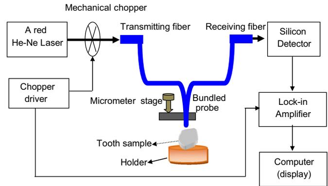
Fig. 1. Schematic diagram of the fiber optic displacement sensor for the detection of stain on human teeth.
