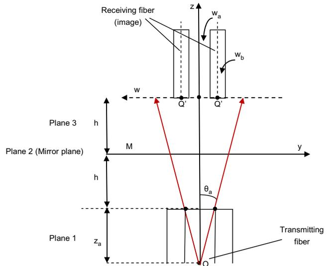
Fig. 3. Cone of light exiting the transmitting fiber.
