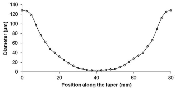
Fig. 5. A tapered fiber with decaying-exponential profile fabricated using a constant hot-zone L<sub>0</sub> = 10 mm.
