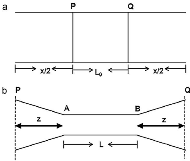
Fig. 4. Shape of a fiber (a) at the beginning (t=0) (b) after tapering (time=t).
