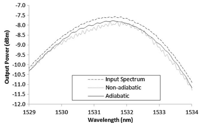
Fig. 13. Output spectra from a microfiber with 10 cm long and  $\sim 3$   $\mu\text{m}$  waist diameter. Input spectrum from EDFA (dashed), adiabatic taper (solid) and non-adiabatic taper (dotted).
