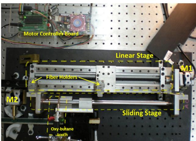
**Fig. 8.** Picture of the fiber tapering Rig assembled in the laboratory. M1 and M2 are the stepper motors of the linear stage and sliding stage respectively.
