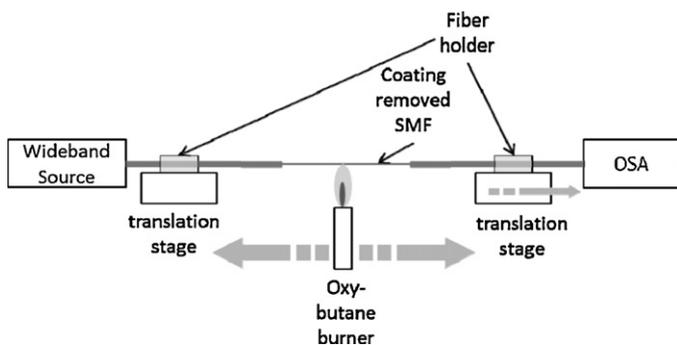
Fig. 11. Schematic illustration of flame brushing technique.
