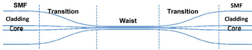
Fig. 1. Typical diameter profile of a tapered fiber.
