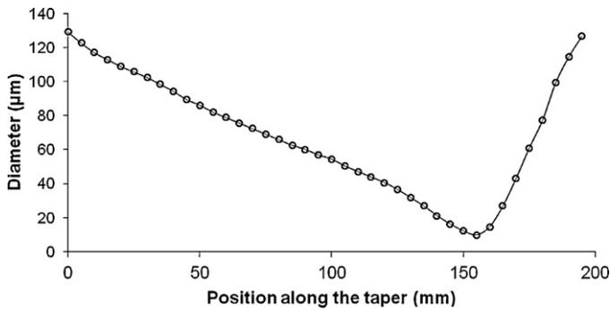
**Fig. 7.** The diameter of tapered fiber is linearly decreasing from  $\sim 128 \mu\text{m}$  to  $\sim 10 \mu\text{m}$  along the 15 cm transition.
