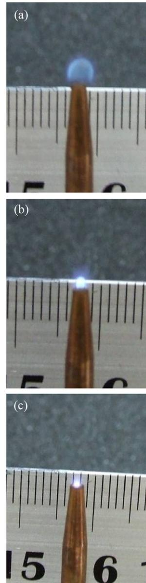
**Fig. 9.** Torch flames at different oxygen supply pressure (a) none (b) equivalent pressure with fuel gas pressure (c) high oxygen.
