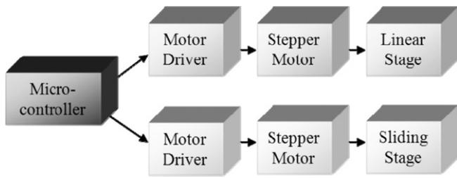
Fig. 10. System diagram of the motor control in the fiber tapering rig.
