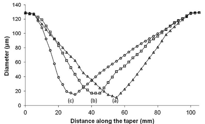
Fig. 6. Three linear taper profiles where the smallest waist point is located at different positions on the tapered fiber. Profile (a) has its smallest waist point at the center of the tapered fiber.
