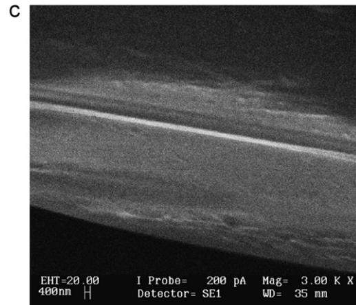
Fig. 12. Characteristic of the fabricated tapered fiber (a) the diameter variation of a biconical tapered fiber fabricated in the laboratory (b) optical microscope image of taper waist, 1.7  $\mu\text{m}$  in diameter (c) SEM image of a 400 nm waist diameter tapered fiber.
