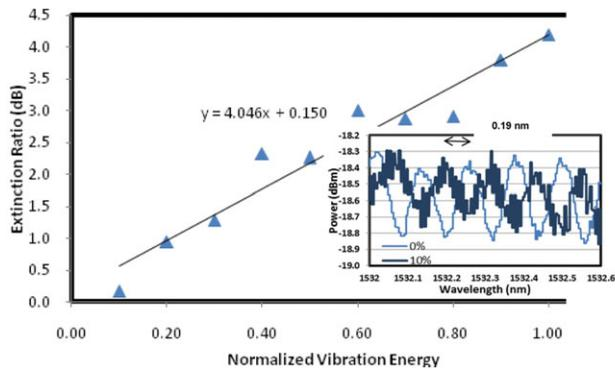
**Figure 4** Extinction ratio against normalized vibration energy. Inset compares the resonant spectrum with and without vibration energy. [Color figure can be viewed in the online issue, which is available at [wileyonlinelibrary.com](http://wileyonlinelibrary.com)]
