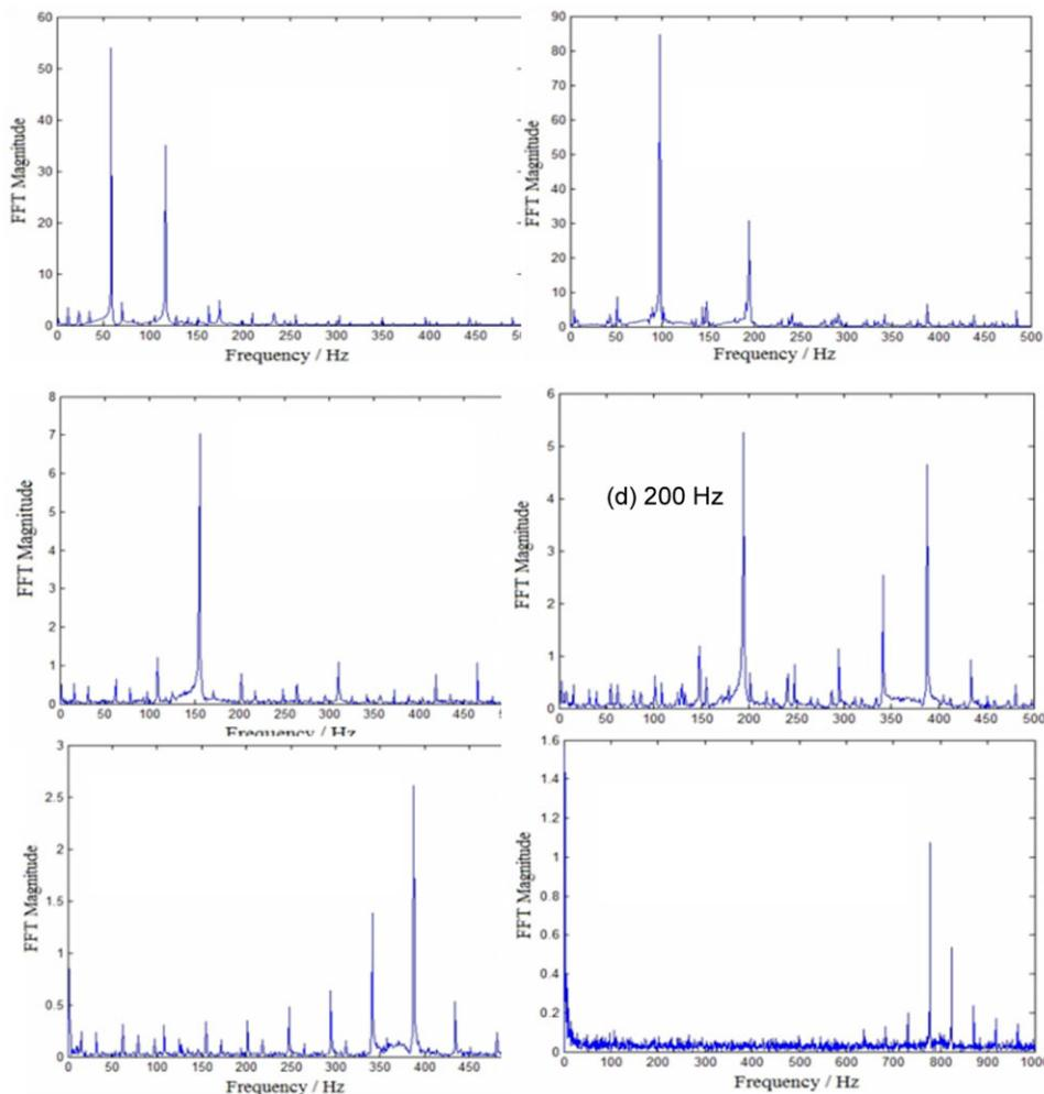
**Figure 5** FFT spectral responses at various vibration frequencies (a) 60 Hz, (b) 100 Hz, (c) 160 Hz, (d) 200 Hz, (e) 400 Hz, and (f) 800 Hz. [Color figure can be viewed in the online issue, which is available at [wileyonlinelibrary.com](http://wileyonlinelibrary.com)]
