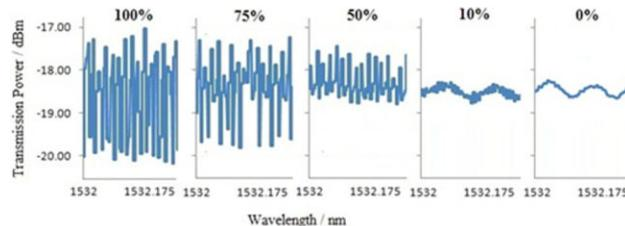
**Figure 3** Resonant spectrum of the MKR at various normalized vibration energy. [Color figure can be viewed in the online issue, which is available at [wileyonlinelibrary.com](http://wileyonlinelibrary.com)]
