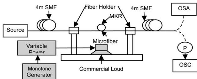
**Figure 1** The schematic diagram of the experimental setup. The microfiber is fabricated through flame brush technique. The MKR loop diameter is 3 mm
