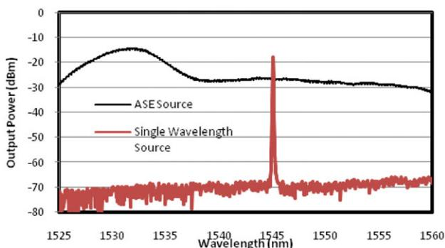
**Figure 2** Output Spectra from both light sources used in this experiment. [Color figure can be viewed in the online issue, which is available at [wileyonlinelibrary.com](http://wileyonlinelibrary.com)]
