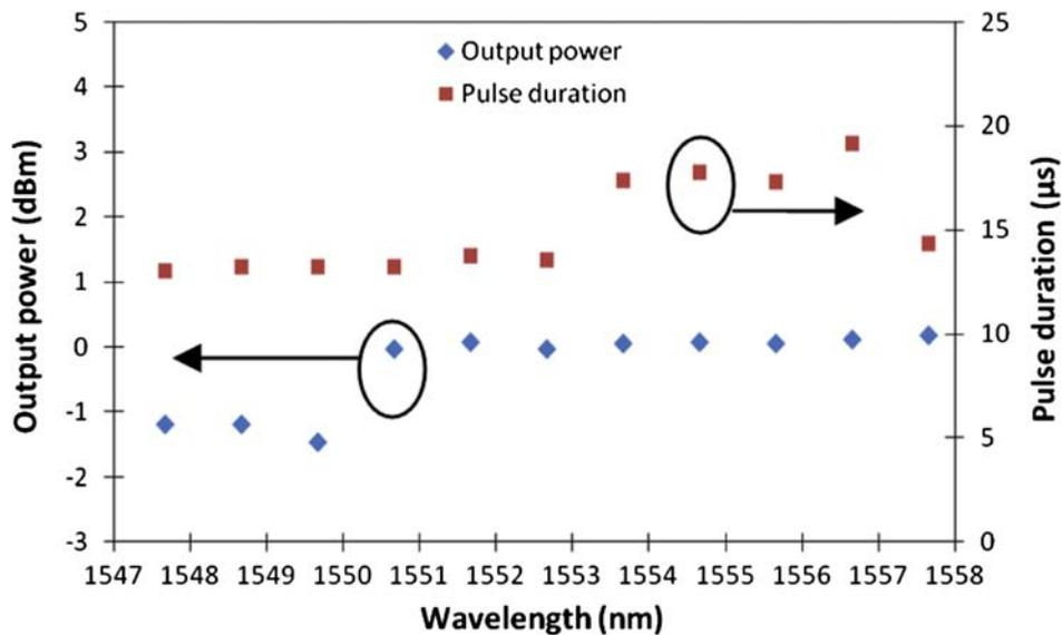
Figure 7. Output power and pulse duration as a function of wavelength. (The color version of this figure is included in the online version of the journal.)
