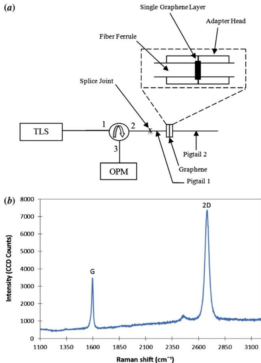
Figure 1. (a) Schematic diagram using an optical extraction forming a graphene layer on the fiber end. The inset shows a blown-up view of the adaptor in which the graphene layer is deposited. (b) The Raman spectrum of graphene flake. (The color version of this figure is included in the online version of the journal.)
