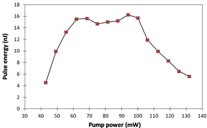
Figure 8. Pulse energy as a function of pump power. (The color version of this figure is included in the online version of the journal.)
