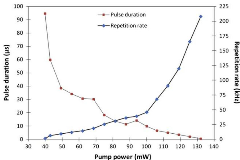
Figure 4. Pulse duration and repetition rate as a function of pump power. (The color version of this figure is included in the online version of the journal.)
