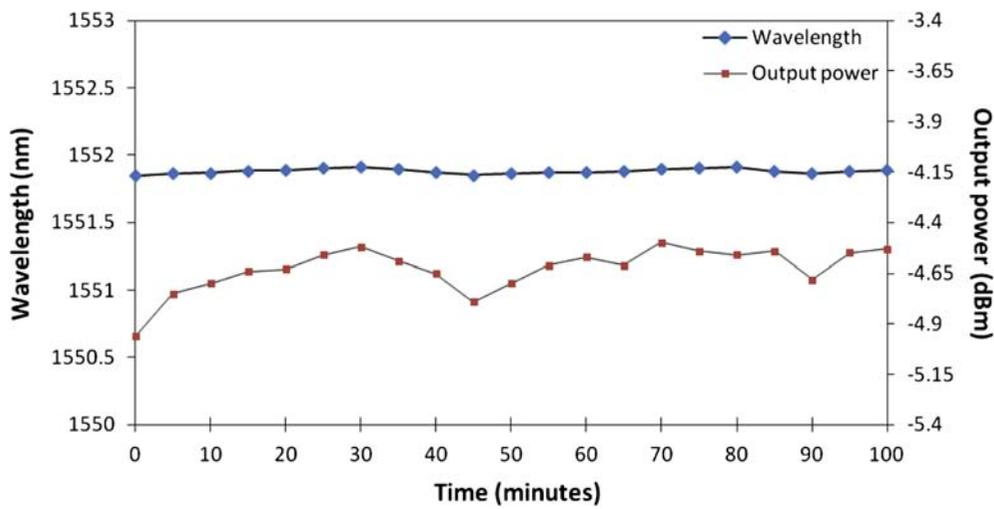
Figure 9. Stability measurement of the output power and wavelength over 100 min observation time. (The color version of this figure is included in the online version of the journal.)
