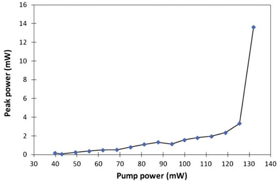
Figure 13. Peak power as a function of pump power. (The color version of this figure is included in the online version of the journal.)
