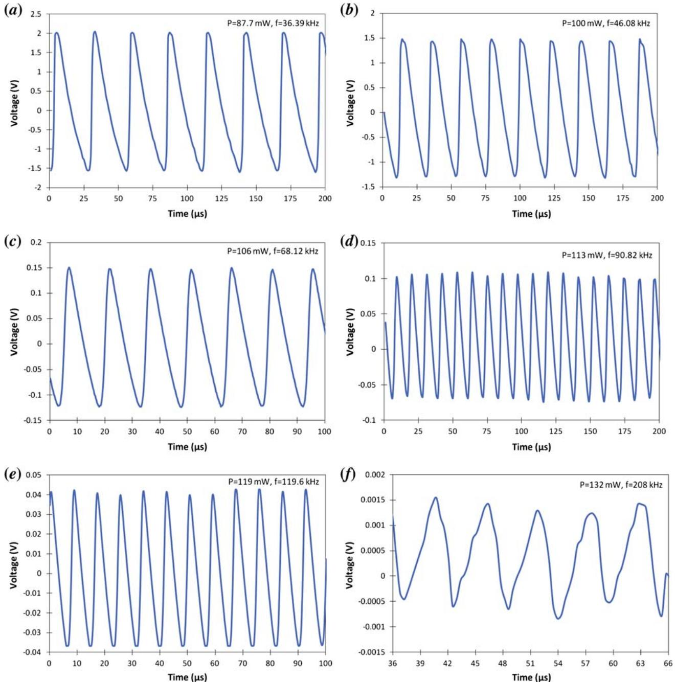
Figure 11. Typical output pulse train of the Q-switched operation under different pump power: (a) 87.7 mW, (b) 100 mW, (c) 106 mW, (d) 113 mW, (e) 119 mW, (f) 132 mW. (The color version of this figure is included in the online version of the journal.)
