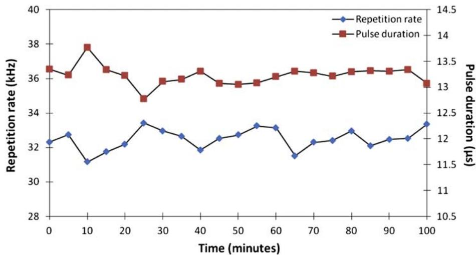
Figure 10. Stability measurement of the repetition rate and pulse duration over 100 min observation time. (The color version of this figure is included in the online version of the journal.)
