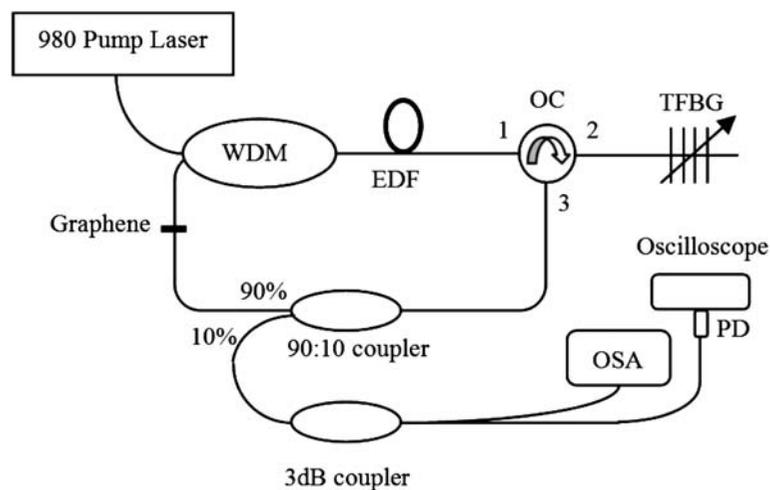
Figure 2. Experimental setup of the proposed graphene-based Q-switched EDFL with a TFBG.
