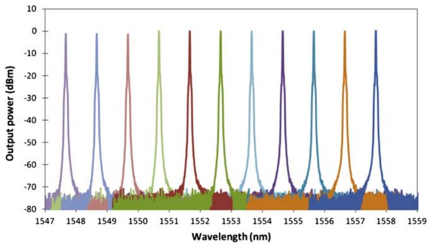
Figure 5. Output spectra of the tunable Q-switched operation for 11 tuned wavelengths. (The color version of this figure is included in the online version of the journal.)
