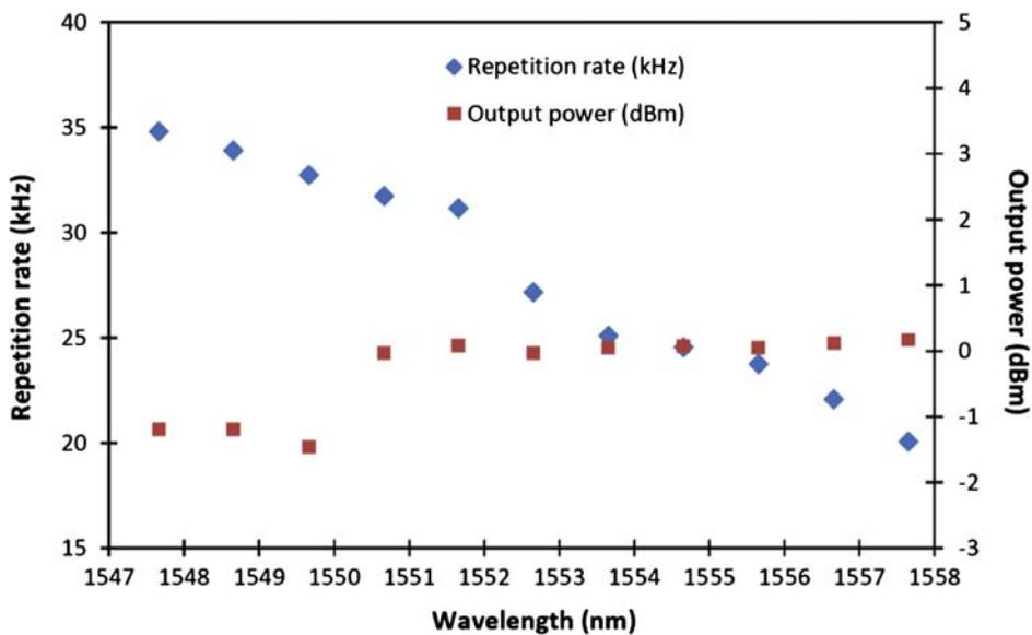
Figure 6. Repetition rate and average output power as a function of wavelength. (The color version of this figure is included in the online version of the journal.)
