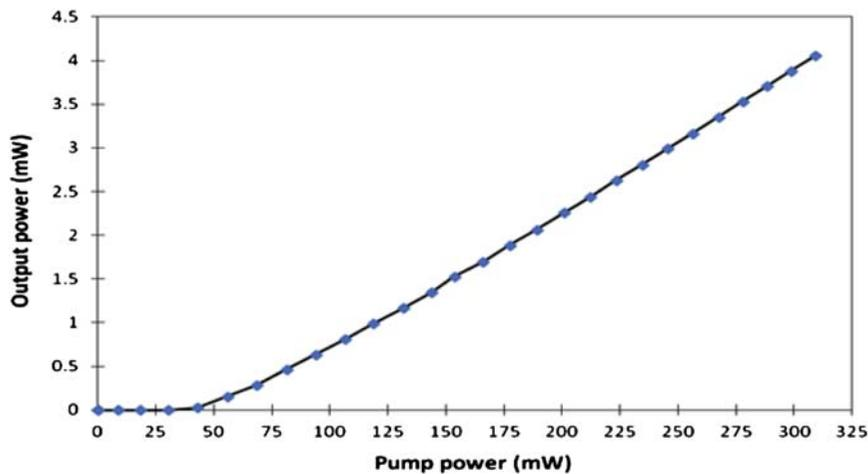
Figure 3. Output power as a function of pump power. (The color version of this figure is included in the online version of the journal.)
