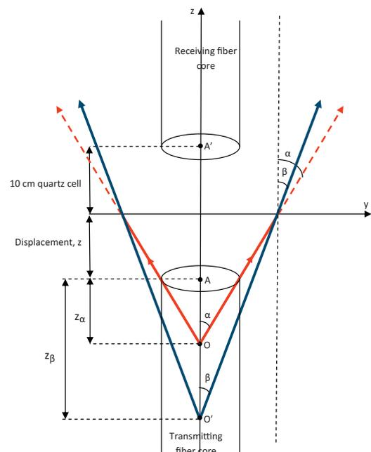
Fig. 4. Cone of light at the transmitting fiber probe.
