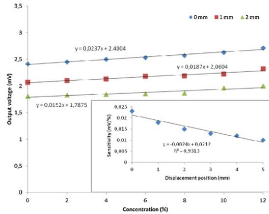
Fig. 3. The output voltage versus concentration of sodium chloride for displacement positions of 0, 1 and 2 mm using the beam-through technique. Inset shows the sensitivity of the salinity sensor versus displacement position.
