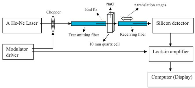
Fig. 1. Schematic diagram for the salinity sensor using beam-through technique with a 10 mm quartz cell path length.
