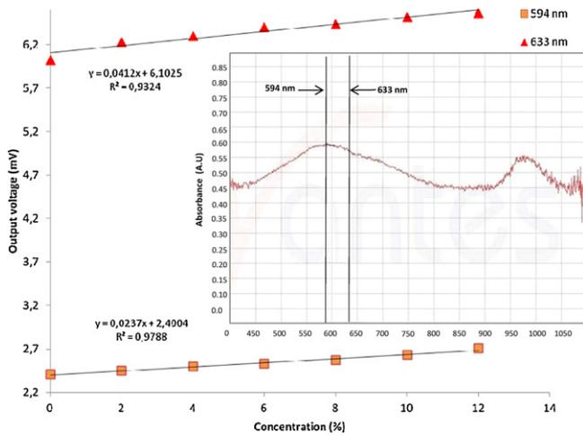
Fig. 5. The output voltage versus concentration of sodium chloride solution using 594 nm and 633 nm He–Ne laser measured at the 0 mm displacement position. Inset shows the absorbance spectrum of a 10% sodium chloride concentration solution.
