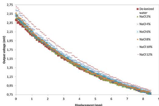
Fig. 2. Output voltage against displacement for various concentrations of sodium chloride in de-ionized water using 594 nm He–Ne laser.
