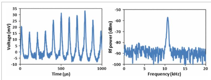
Fig. 3. Temporal characteristic of the proposed multi-wavelength Q-switched BEFL with a channel spacing of 0.086 nm. (a) Oscilloscope trace. (b) RF spectrum.
