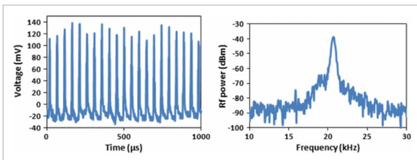
Fig. 5. Temporal characteristic of the proposed multi-wavelength Q-switched BEFL with a channel spacing of 0.173 nm. (a) Oscilloscope trace. (b) RF spectrum.
