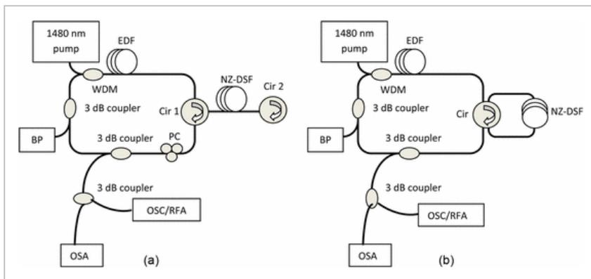
Fig. 1. Experimental set-up of the proposed multi-wavelength BEFL configured with (a) single BS and (b) double BS.
