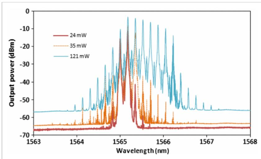
Fig. 4. Output spectra of the BEFL configured with a double BS at various 1480 nm pump power when the BP power is fixed at 5.4 dBm.
