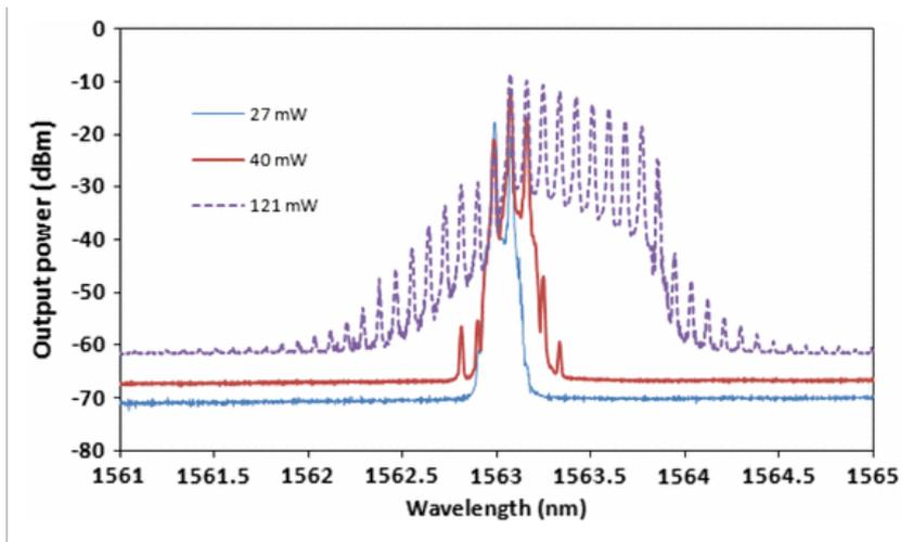
Fig. 2. Output spectra of the BEFL configured with a single BS at various 1480 nm pump power when the BP power is fixed at 5.4 dBm.
