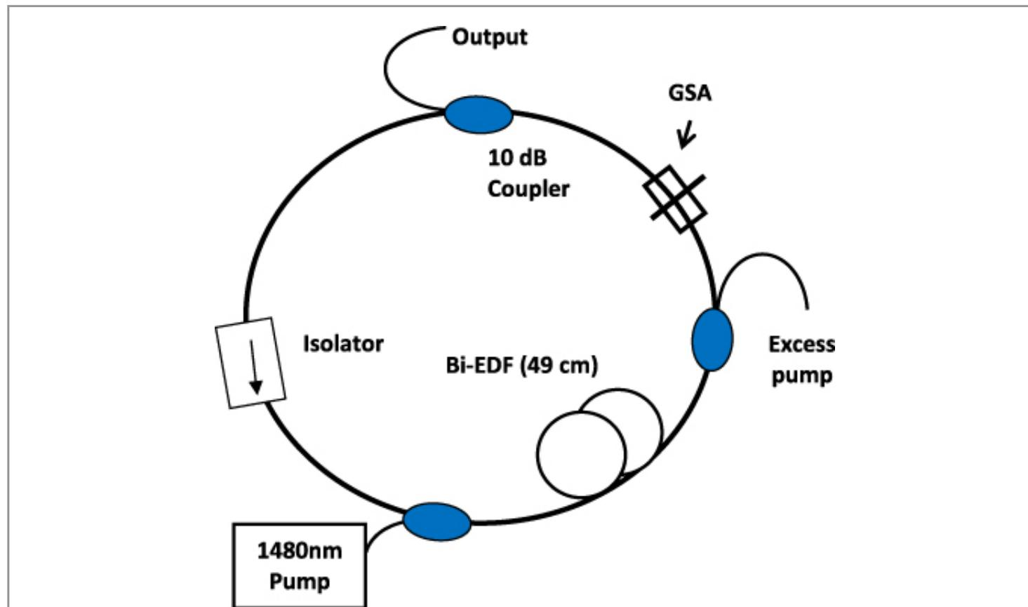
**Figure 1.** Experimental setup of the proposed graphene based *Q*-switched EDFA.
