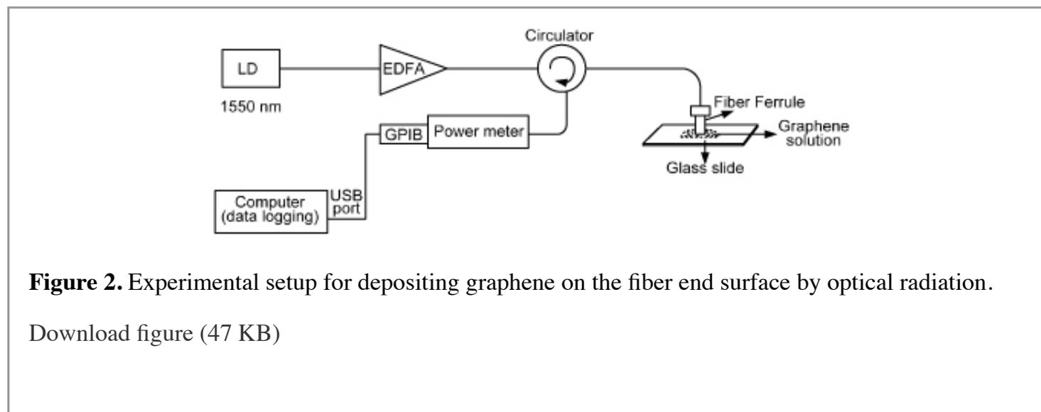
**Figure 2.** Experimental setup for depositing graphene on the fiber end surface by optical radiation.
