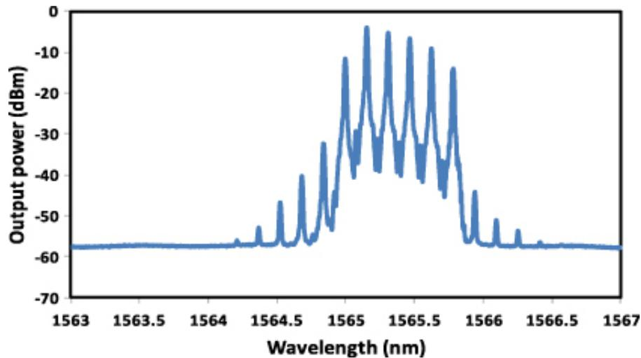
**Figure 2.** Output spectrum of the MWBEFL with a double Brillouin spacing.
