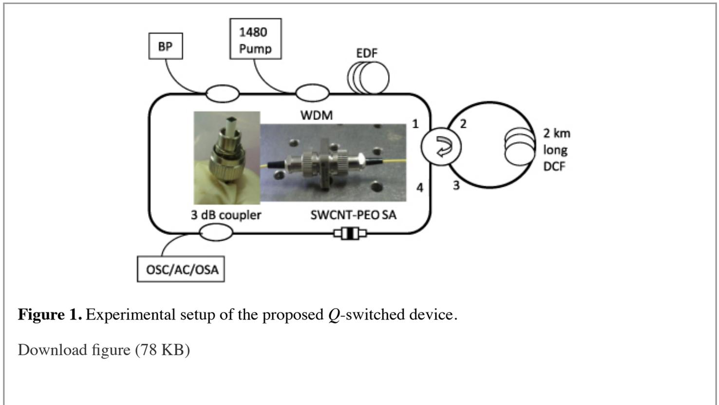
**Figure 1.** Experimental setup of the proposed *Q*-switched device.
