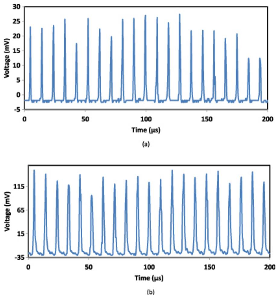
**Figure 3.** Output pulses train from the *Q*-switched lasers (a) without and (b) with the BP.
