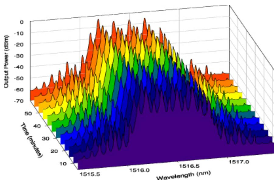
**Figure 5.** Stability measurement of random laser output with angled cleaved ends, taken for a period
