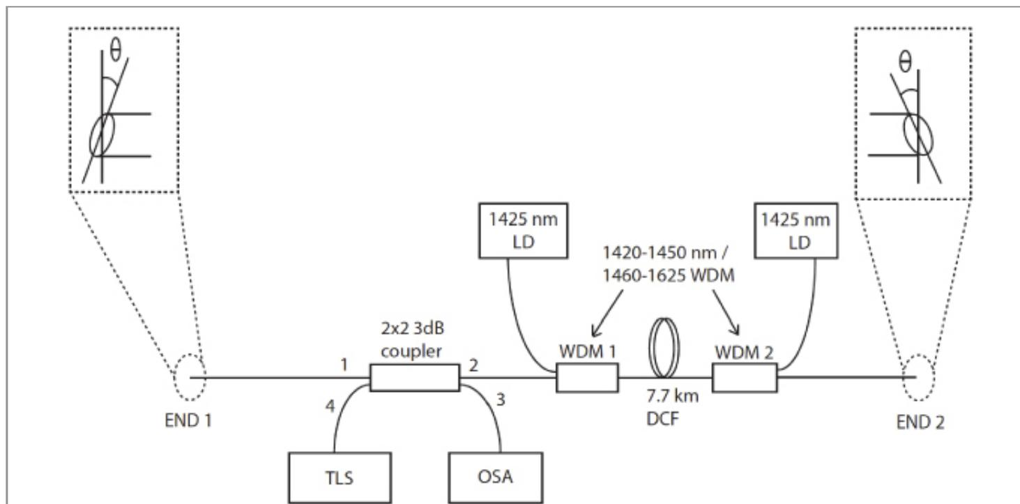
**Figure 1.** Experimental setup for the S-band multi-wavelength Brillouin–Raman distributed feedback random fiber laser; angle of the fiber cleave at both ENDS 1 and 2 are  $\sim 8^\circ$ .
