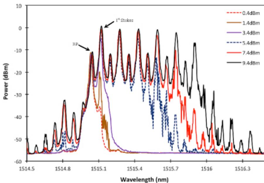
**Figure 3.** Output spectrum of the S-band distributed feedback BRRFL with angle-cleaved fiber ends at different BP powers.
