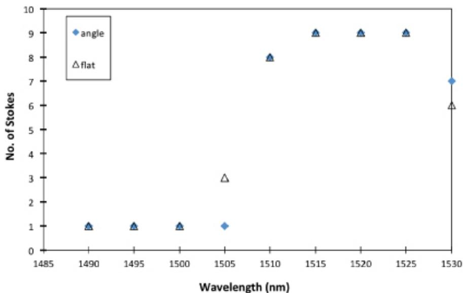
**Figure 4.** The number of Brillouin Stokes lines generated against different BP wavelength for flat and angle-cleaved fiber ends.
