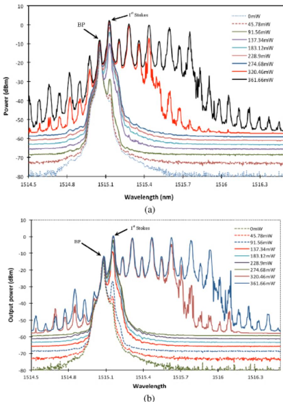
**Figure 2.** The output spectrum of the S-band BRRFL for different Raman pumping power using (a) flat-cleaved fiber ends, and (b) angle-cleaved fiber ends.
