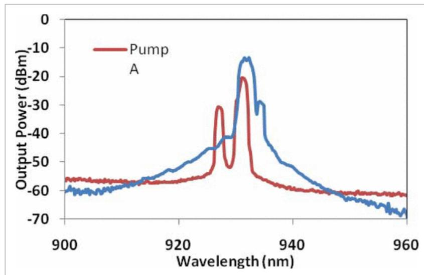
Fig. 5. Output spectra of two different 931-nm pump sources used in the experiment.
