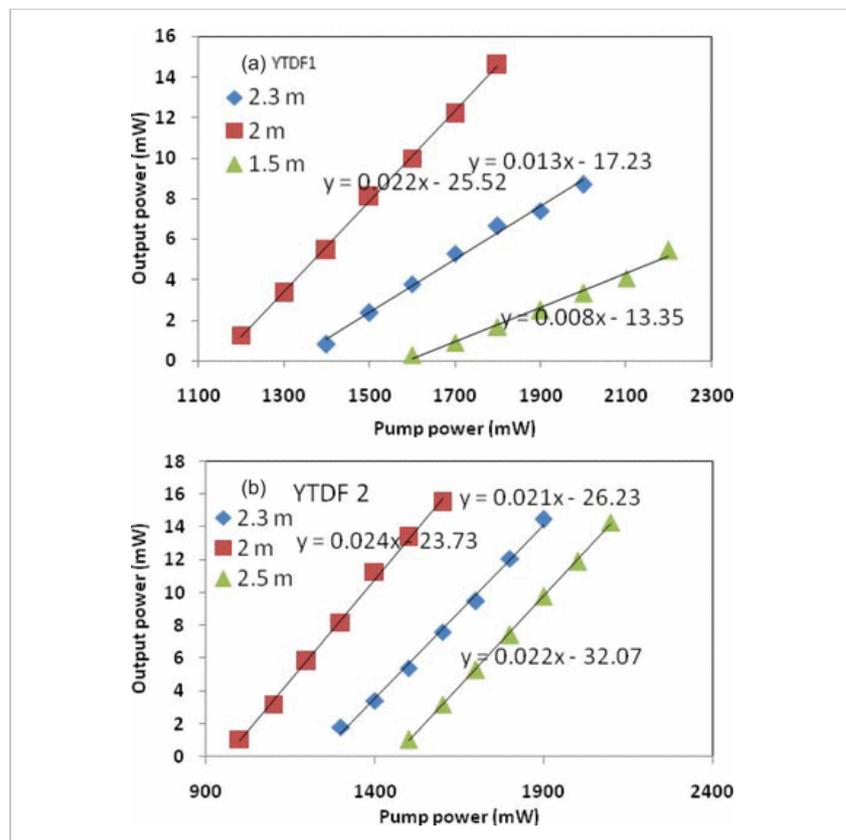
Fig. 3. Output power of the proposed YTFL against the pump power at different YTDF lengths using (a) YTDF 1 and (b) YTDF 2 samples as the gain medium.
