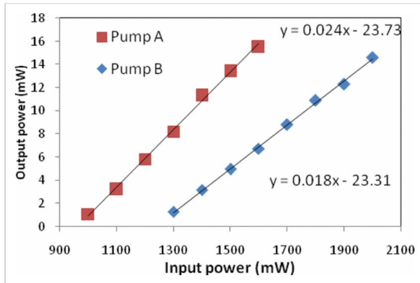
Fig. 6. Output power against pump power characteristics for the proposed YTFL with two different pump sources.
