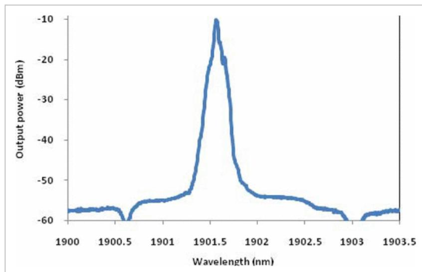
Fig. 4. Output spectrum of the YTFL with YTDF 2 in conjunction with 931-nm pumping.
