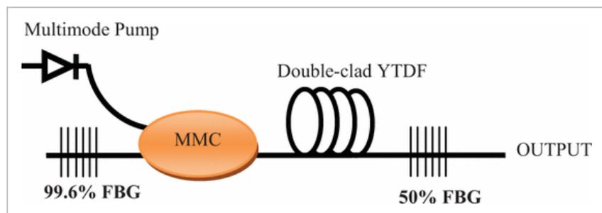
Fig. 1. Configuration of the proposed TYDFL.
