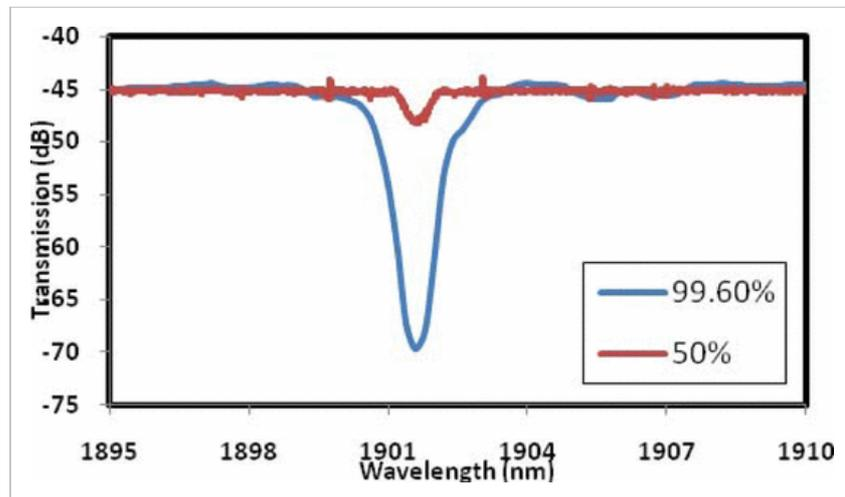
Fig. 2. Transmission spectrum of both FBGs used in the laser cavity.
