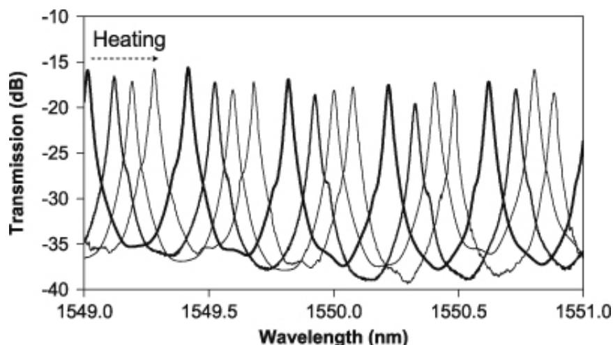
**Figure 2.** Transmission profile of the microring filter at different temperatures.
