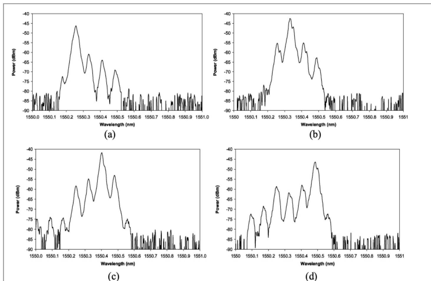
**Figure 4.** Brillouin fibre spectra after the microring filter with the extraction of (a) the Brillouin pump and (b)–(d) the first, second and third Stokes lines, respectively.
