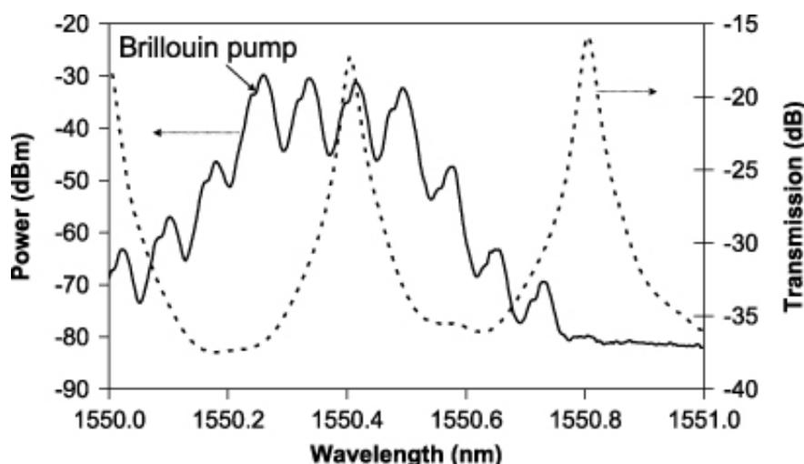
**Figure 3.** Brillouin fibre laser spectrum with the Brillouin pump and three adjacent Stokes with a
