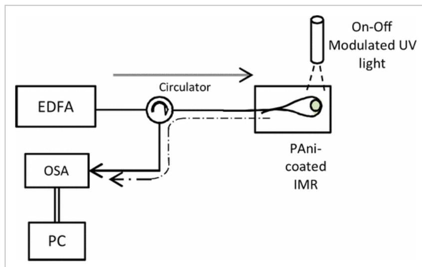
Fig. 5. Experimental setup of the proposed UV detector.
