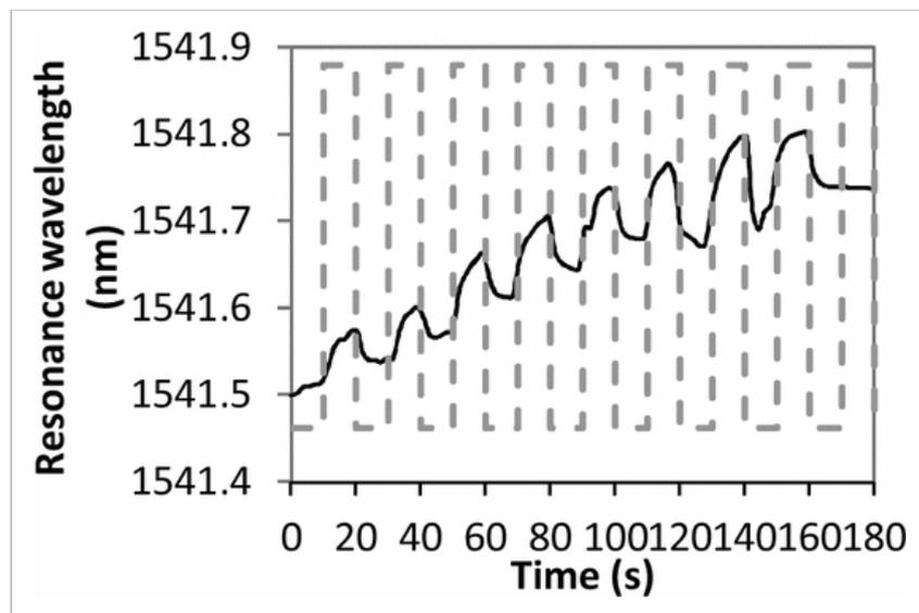
Fig. 7. Resonance wavelength responses to the exposure of UV light for on and off states at different exposure distance or power.
