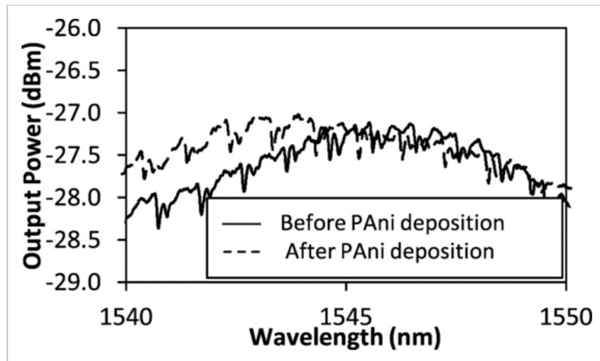
Fig. 4. Output spectra of the UV detector. Solid: before deposition of PAni. Dotted: after deposition of PAni.
