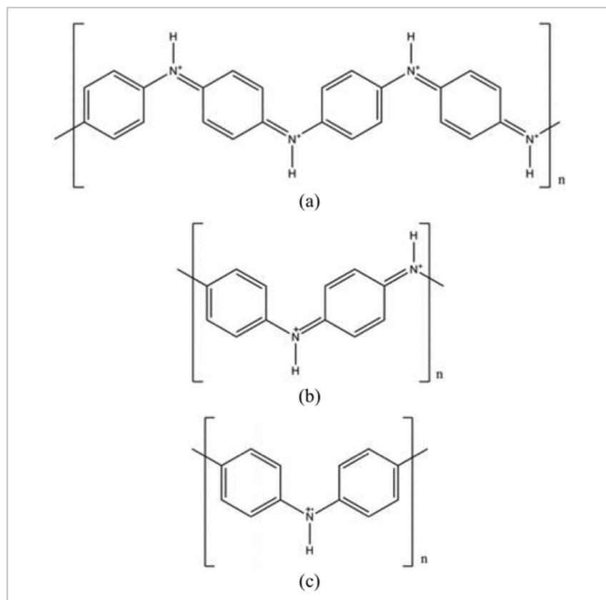
**Fig. 1.** Chemical structure. (a) General PANi and PANi in both (b) quinoid, and (c) benzenoid forms.
