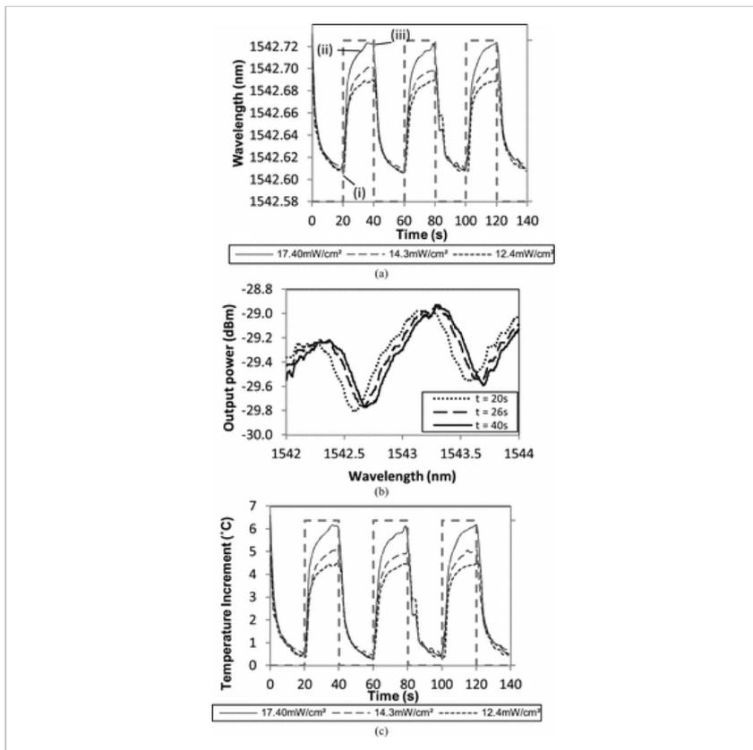
**Fig. 6.** (a) Resonance wavelength responses of the detector to on-off UV light of different light intensities: 12.4, 14.3, and 17.40  $\text{mW}/\text{cm}^2$ . (b) Output spectra of the detector for UV light intensity of 17.4  $\text{mW}/\text{cm}^2$  during "on" state. (c) Calculated temperature increment at the detector.
