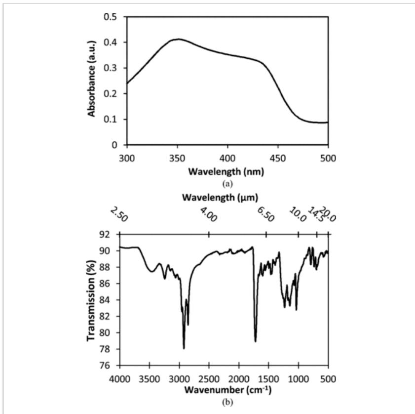
Fig. 2. Chemical structure determination of PANi. (a) UV absorbance. (b) FTIR spectrum.
