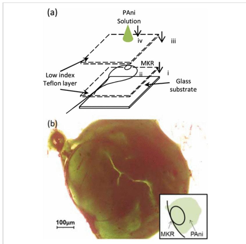
**Fig. 3.** (a) Fabrication steps of the proposed detector. Sequence is stated by the Roman numbers. (b) Microscope image of an MKR coated with a thin layer of PANi. There is a thin layer of low index Teflon in between PANi layer and MKR to prevent light in MKR from total leakage loss into the PANi. Inset: illustration of the proposed detector.
