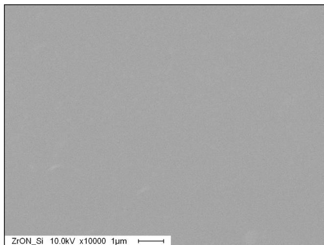
Fig. 1. Typical FESEM micrograph of a ZrON/Si film prepared at 700 °C.
