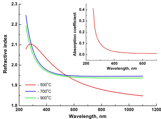
**Fig. 3.** Dispersive refractive index  $n(\lambda)$  in ZrON/Si thin films prepared at different temperatures.
