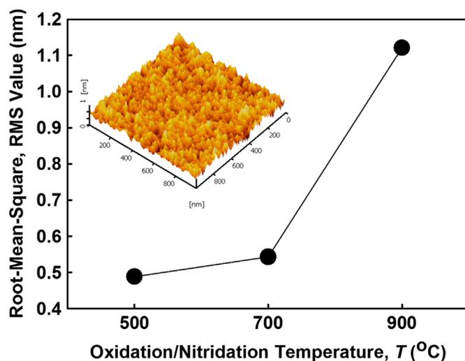
Fig. 2. The RMS value of investigated samples as a function of oxidation/nitridation temperature. The inset shows three-dimensional AFM topography of the sample treated at 700 °C.
