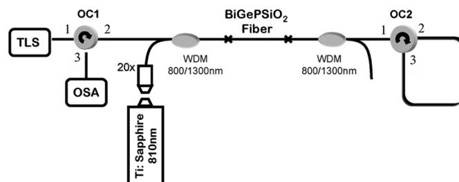
Fig. 1. Experimental setup of Bismuth-doped fiber amplifier in a double-pass configuration.
