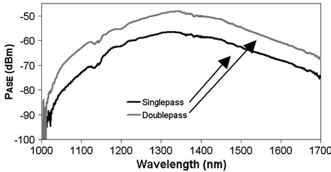
Fig. 2. ASE spectra of single- and double-pass BDFA.
