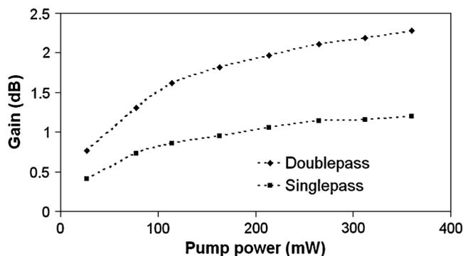
Fig. 5. Signal gain against input pump power of the BDFA.
