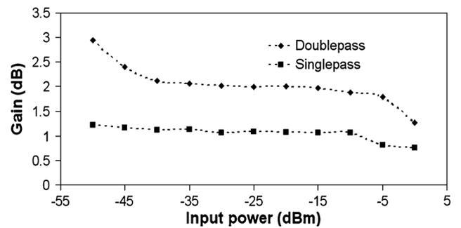
Fig. 4. Signal gain of the single- and double-pass BDFAs at different input powers.
