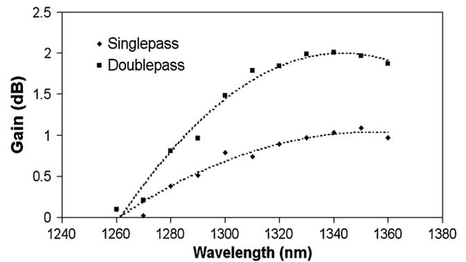
Fig. 3. Signal gain for single- and double-pass BDFAs at different signal wavelengths.
