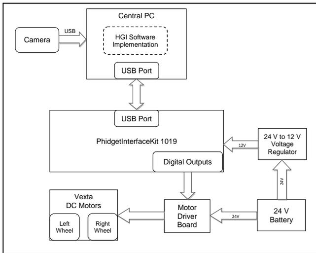
**Fig. 9.** Block diagram of EPW hardware configuration.
