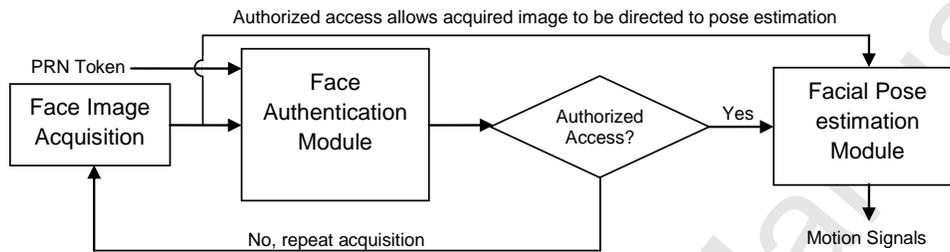
**Fig. 1.** Block diagram of the software implementation of HGI.
