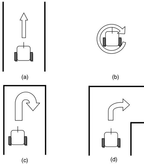
**Fig. 17.** Basic motions to pilot electrical wheelchair: (a) Forward (b) On-the-spot turn (c) U-turn (d) Corner turn.
