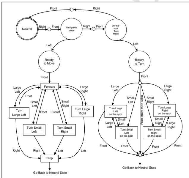
**Fig. 7.** State transition diagram used by MPG to pilot electrical wheelchair.
