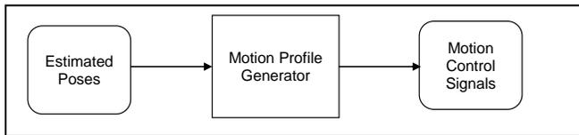
**Fig. 6.** Input and output of MPG.
