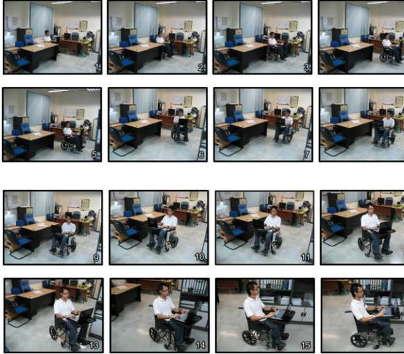
**Fig. 19.** A series of navigation sequences using HGI control in a simple maze-type environment.
