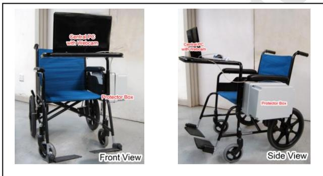
**Fig. 8.** EPW Prototype for HGI deployment.
