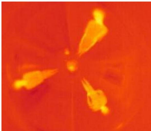
Fig. 19: Thermal image with temperature range 20°C to 40°C used for detecting trespasser.
