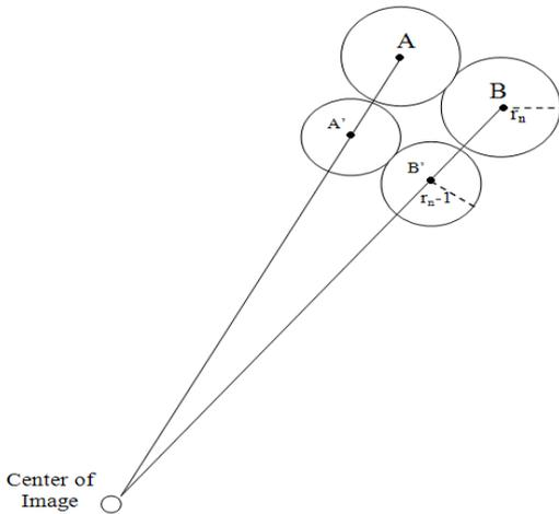
Fig. 6: Circular Sampling Structure in Log-Polar Mapping.
