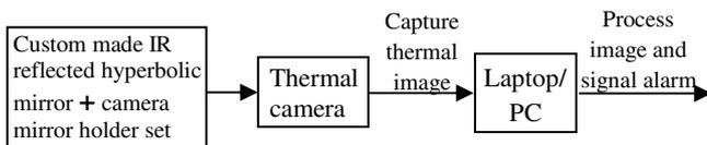
Fig. 1. Omnidirectional Thermal Imaging System Model
