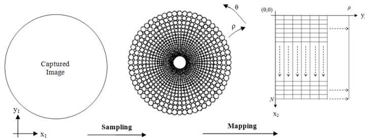
Fig. 5: A graphical view of log-polar mapping.
