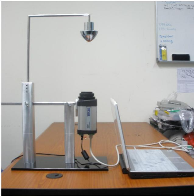
Fig.4: Overall fabricated omnidirectional imaging system model
