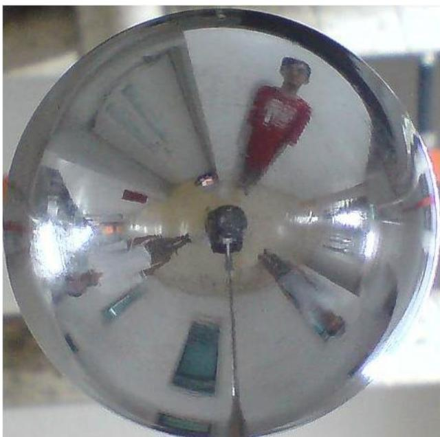
Fig. 16: Omnidirectional digital color image on the site for trespasser detection.
