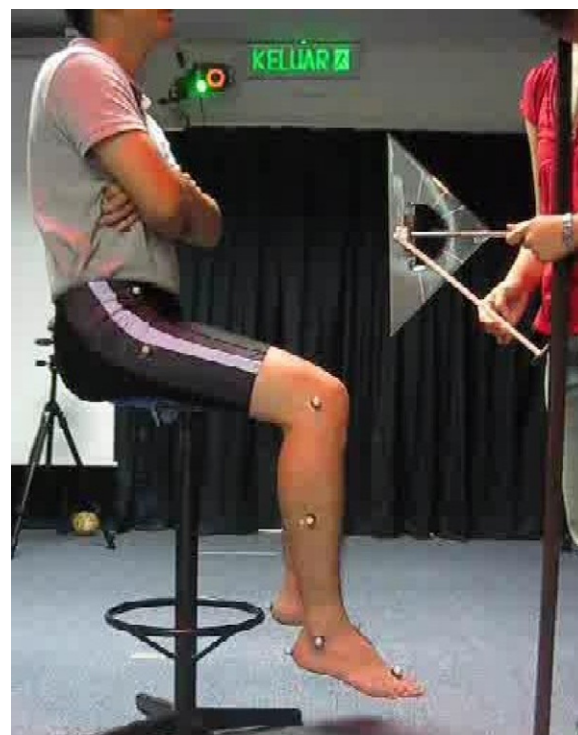
Fig. 1. Experimental setup for reflex assessment tests. The subject sits on a high stool with both feet not touching the ground. The patellar tendon of each leg is tapped using a Queen square reflex hammer. The Queen square reflex hammer is first raised to a certain angle measured using an attached protractor. The hammer is then released to tap on the patellar tendon. The experiment is recorded by the motion analysis system Nexus 1.3.
