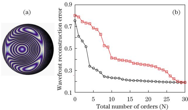
Fig. 3. (a) Wavefront contour map of the function described in Eq. (24) and (b) wavefront reconstruction error as a function of the total number of orders.
