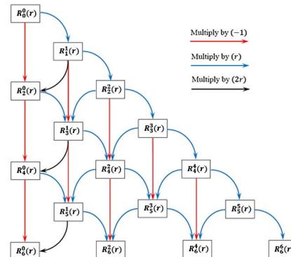
Fig. 1. Flow of proposed method to compute Zernike radial polynomials  $R_n^m(r)$ .
