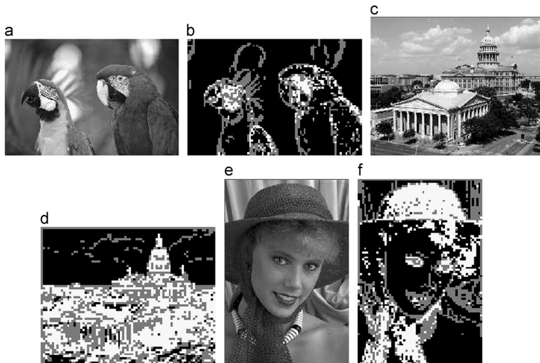
Fig. 7. Block classification output of “parrots”, “churchandcapitol” and “womanhat”. Image (a), (c) and (e) on the left are the luminance level of the original images, while images (b), (d) and (f) on the right are the corresponding 8 × 8 block classification output. The plain, edge and texture blocks are represented by black, gray and white colors respectively. The ratios of the plain (P), edge (E) and texture (T) blocks of these images are shown in Table 2.
