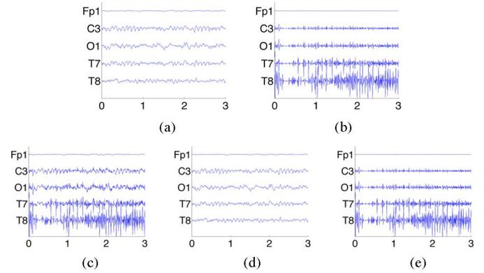
Fig. 3. Sample of EEG and artifact before, during, and after artifact removal. (a) *ReferenceEEG*. (b) *ReferenceArtifact*. (c) *EEG + Artifact*. (d) *ProcessedEEG*. (e) *RemovedArtifact*.
