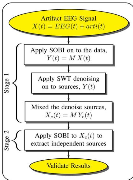
Fig. 2. BSS-wavelet algorithm to enhanced independent components.
