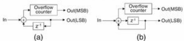
Figure 1 Kotoulas and Andriadis' basic filter structures. a Feedback type; b Feedforward type.
