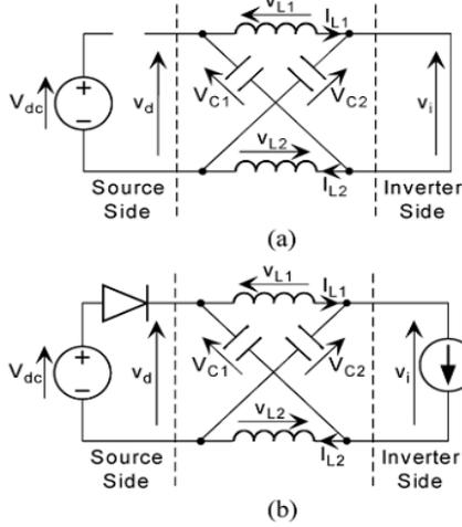
Figure 2. Equivalent Z-source inverter circuits in (a) shoot-through state (b) non-shoot-through state [3].
