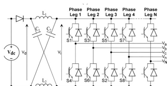
Figure 3. General structure of a Z-source converter [3]
