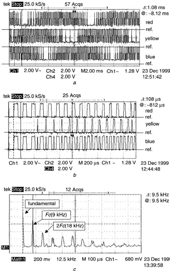
Fig. 6 Three-phase PWM switching scheme at modulation index 0.5
