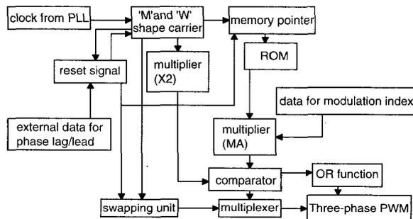
Fig. 4 Overall block diagram of three-phase PWM modulator
