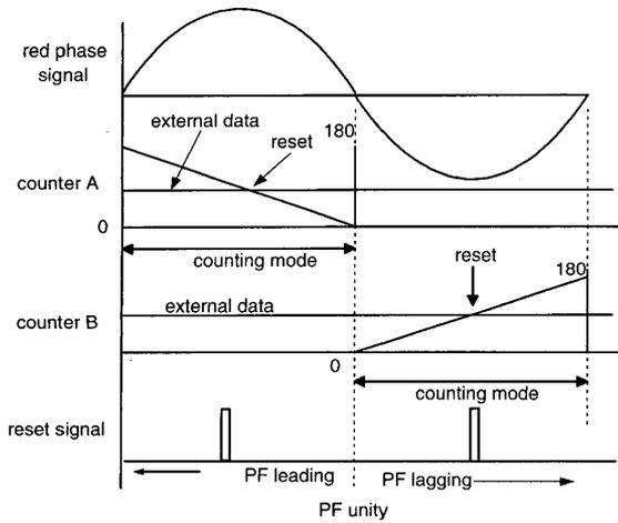
Fig. 5 Operation of reset signal for phase shift
