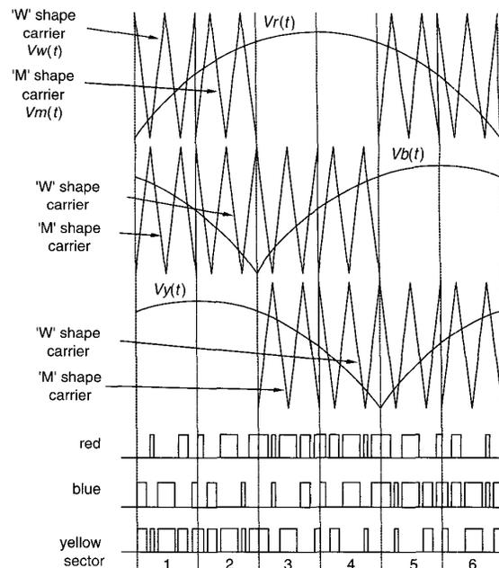
**Fig. 2** Method of generating three-phase PWM switching scheme
