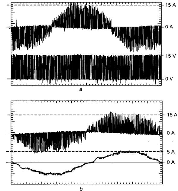
Fig. 7 AC current at modulation index 0.5
