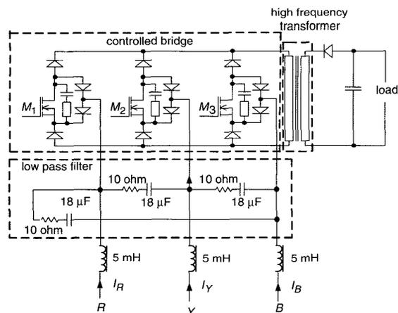
**Fig. 1** Flyback converter with three devices controlled bridge topology and isolation transformer
