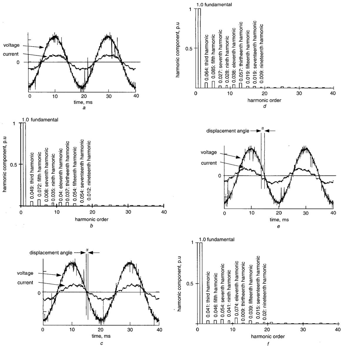
**Fig. 8** Effect of shifting PWM pattern on operating power factor
