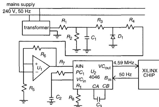
Fig. 3 Phase locked-loop circuit
