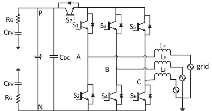
Fig. 1. H7 topology for three-phase transformerless PV systems.
